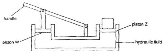
Which change will result in the heaviest load being lifted with the same force applied at the handle?
