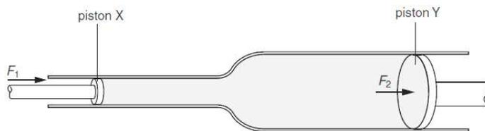
The force  $F_1$  of the driver's foot on the brake pedal moves piston X. The space between pistons X and Y is filled with oil which cannot be compressed. The force  $F_2$  exerted by the oil moves piston Y. This force is applied to the brake mechanism in the wheels of the car.
